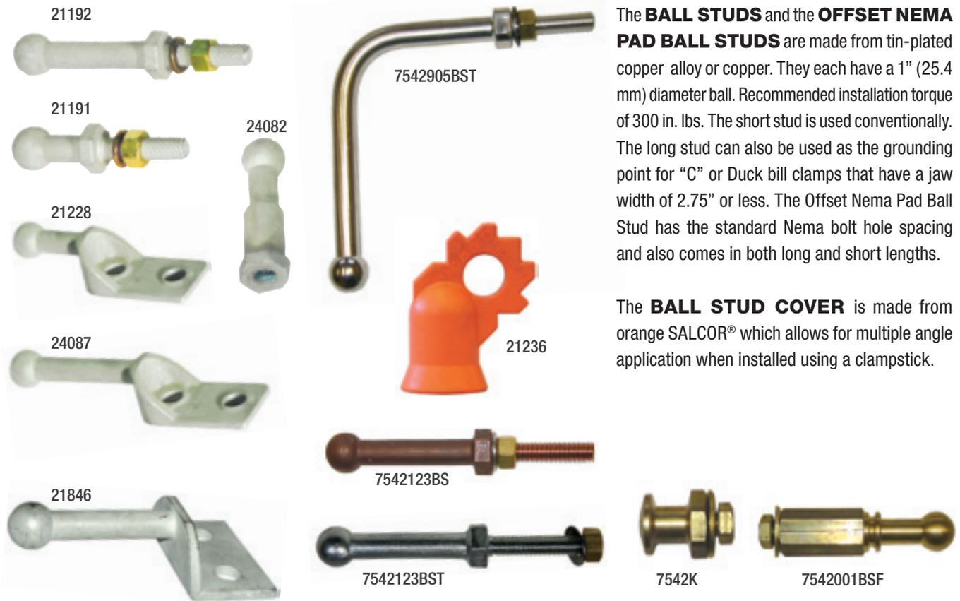
The **BALL STUDS** and the **OFFSET NEMA PAD BALL STUDS** are made from tin-plated copper alloy or copper. They each have a 1" (25.4 mm) diameter ball. Recommended installation torque of 300 in. lbs. The short stud is used conventionally. The long stud can also be used as the grounding point for "C" or Duck bill clamps that have a jaw width of 2.75" or less. The Offset Nema Pad Ball Stud has the standard Nema bolt hole spacing and also comes in both long and short lengths.
