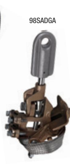
The **JUMPER HEADS** have a maximum opening of 19/16” (4.0 cm) and are designed with built-in universal joints in order to accommodate installation lines at an angle. The jumper heads have a quick action tightening screw for fast closing. Threaded adapters are used to accept 5/8-11 threaded non-shrouded ferrules. A hose clamp is included for connection strain relief.
