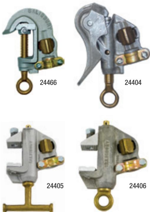
These **DUCKBILL** and **"C" CLAMPS** feature pressure terminations for use with plain ferrules. Made of high strength aluminum with bronze eye-screws, these Grade 5 clamps are designed for smooth operation and long service life. Use Duckbill clamps for all grounding applications from .16 to 1.1" diameter and "C" clamps for all grounding applications from .06 to 1.26" diameter.
