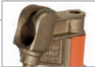
The **BALL AND SOCKET GROUNDING SYSTEM** allows for variable angle accessibility. This system is compact and lightweight. There are fixed grounding points on the socket clamp. The 21190 Socket Clamp, made from bronze alloy, has a socket size of 1 inch (25.4 mm) and a threaded bore boss of 5/8"-11 UNC. The socket clamp has an integral cable support with strain relief sleeve.
