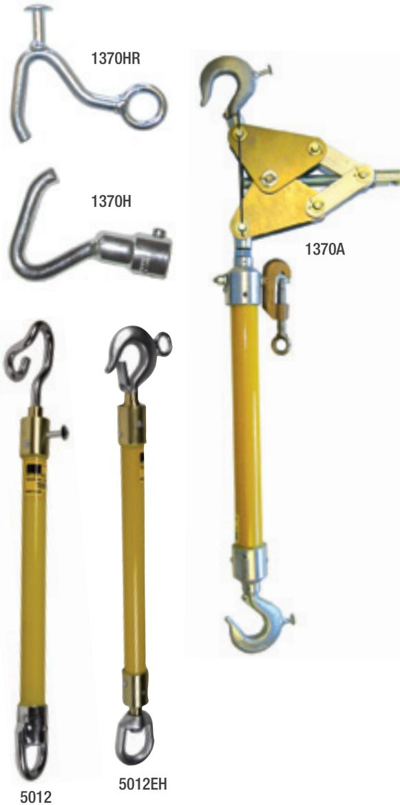
The **SECTIONALIZER KIT** temporarily disconnects and isolates a section of line without interrupting service to the balance of the circuit. The entire operation of installation and removal of the sectionalizers can be performed with live line tools. Particularly useful when circuits are interrupted as a result of conductor, insulation or pole failures. Service can be restored by cutting in sectionalizers to isolate the section of line that is in trouble.
